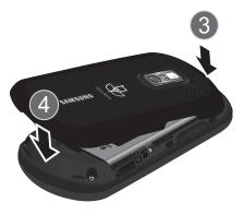
Press along the entire edge of the cover to verify it is securely in place.
